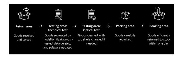
Over the years we have broadened the refurbishment solution's scope to include additional router models, media receivers, business routers, and mesh repeaters. Our software platform and model-independent test boxes allow the rapid extension of test scenarios to new device models within three weeks. Notably, device manufacturers seldom provide test software or specify pass/fail criteria, leaving us to define and establish these crucial parameters in close collaboration with Deutsche Telekom.
